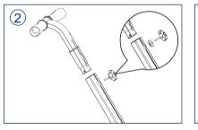
Insert handlebar into leansteer frame, and fasten the height adjuster nut.
