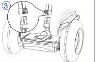
Insert leansteer frame into main frame, and fasten the clockwise joint.
